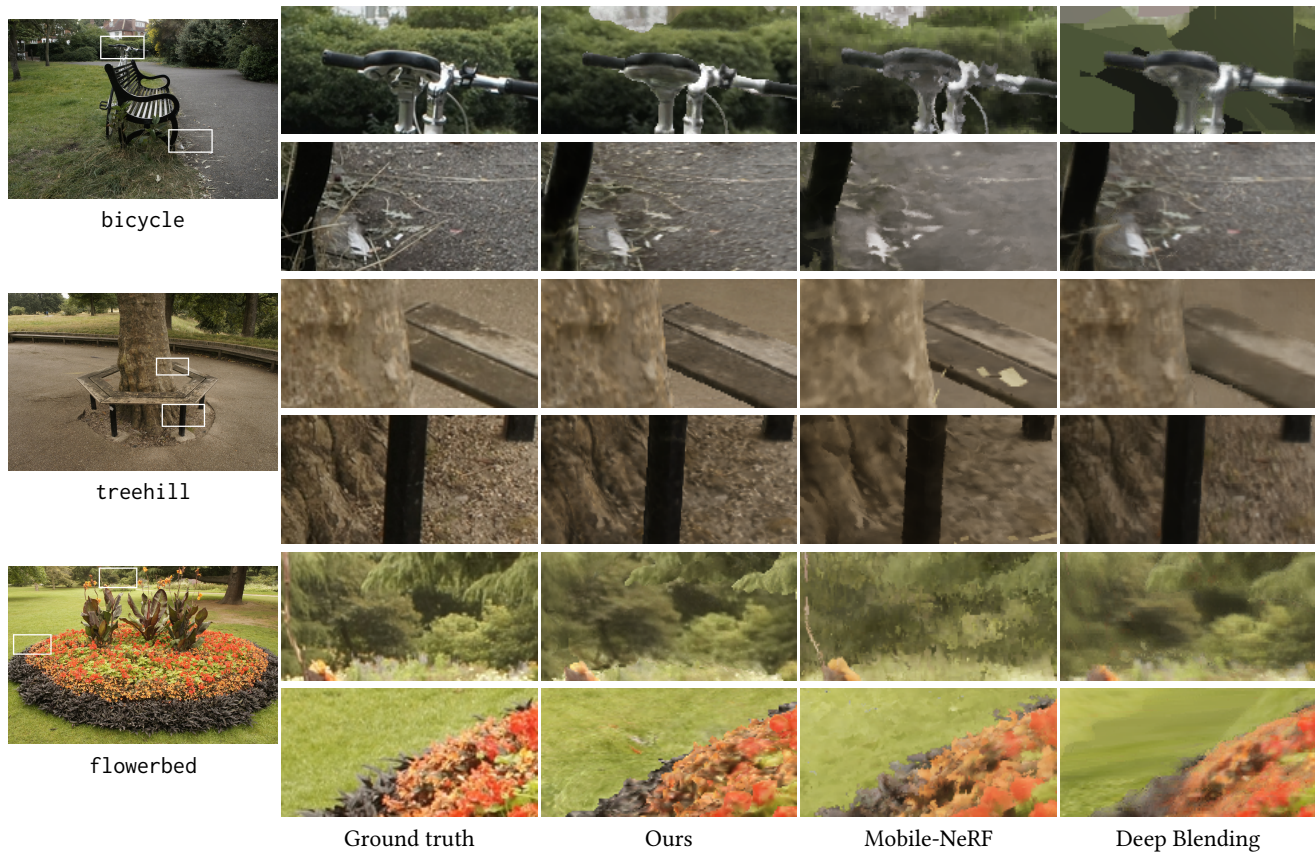
Figure 4: Test-set renderings (with insets) for our model and the two state-of-the-art real-time baselines we evaluate against, using scenes from the mip-NeRF 360 dataset. Deep Blending [Hedman et al. 2018] produces posterized renderings when the proxy geometry used as input is incorrect (such as in the background of the bicycle scene) and renderings from MobileNeRF [Chen et al. 2022a] tend to exhibit aliasing artifacts or oversmoothing.
