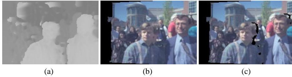
Figure 4: Results of multi-view stereo algorithm: (a) depth estimate for first frame; (b) warped (resampled) images without visibilities; (c) with visibility computation.
