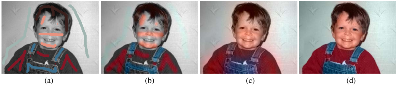
Figure 1: Piecewise smooth color interpolation in a colorization application: (a) input gray image with color strokes overlaid; (b) solution after 20 iterations of conjugate gradient; (c) using 1 iteration of hierarchical basis function preconditioning; (d) using 1 iteration of locally adapted hierarchical basis functions.
