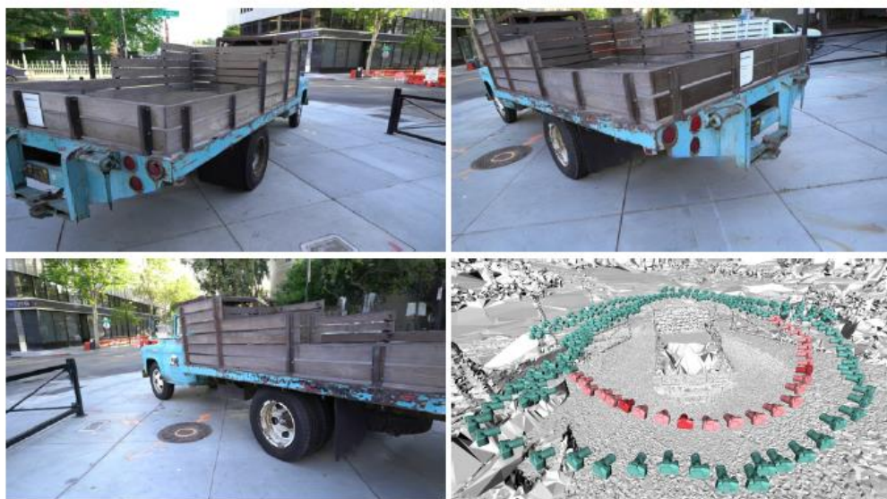
Fig. 1: Novel view synthesis from unstructured input images. The first three images show our synthesized results on the Truck scene from Tanks and Temples [21]. The unstructured image sequence was recorded using a handheld cam-
