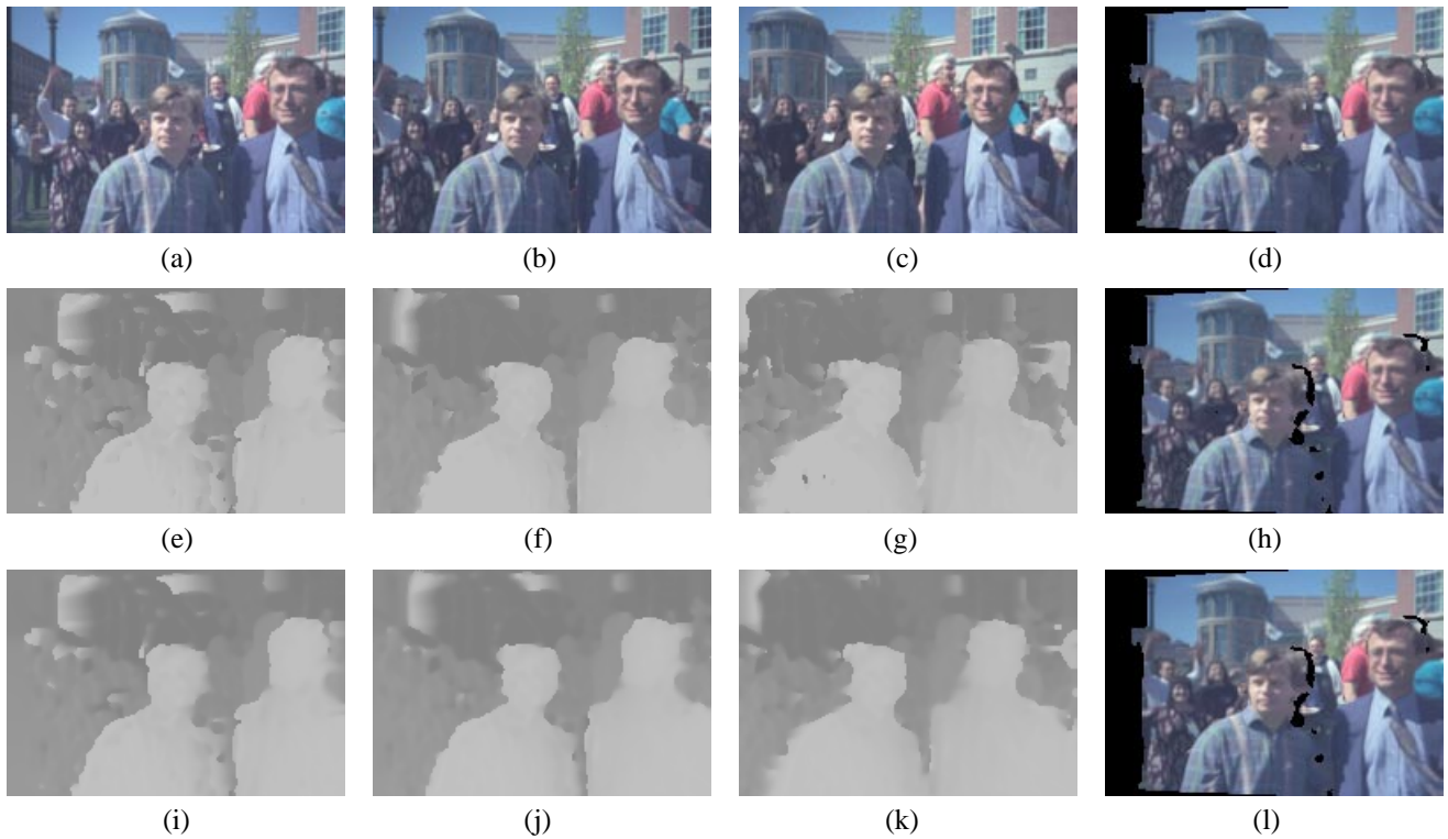
Figure 3. Results on the symposium sequence: (a–c) first, third, and fifth (last) frame; (e–g) initial depth estimates; (i–k) refined (multi-view) depth estimates. Warped (resampled) images: (d) after initial estimate; (h) with visibility computation; (l) with refined estimates.
