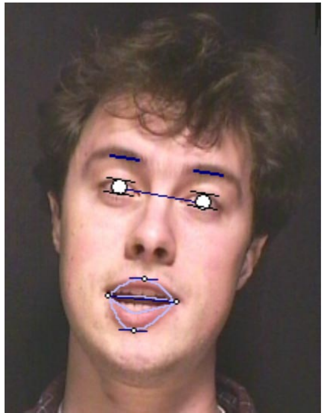
Figure 4 A frame of video tracked by our system. The ten scalar quantities sent to the renderer are easily derived from the features detected by our tracker.
