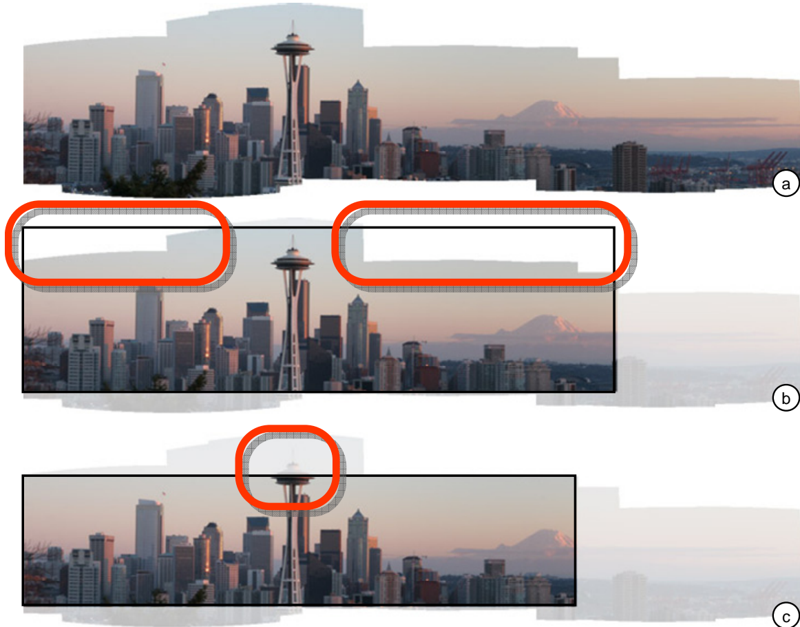
Figure 1: Common mishap when taking panoramas: (a) The user is trying to cover the Seattle Space Needle, but does not cover enough of the sky around it. During cropping, the user has the choice between (b) including white fringes and (c) cropping relevant content.
