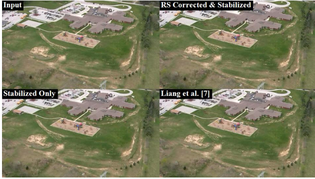
Figure 5. A Qualitative Comparison: One frame from the video skool.mp4 . We compare the output of our algorithm (top right) with the result of naive stabilization (bottom left) and the result obtained with the algorithm described in [7] (bottom right).
