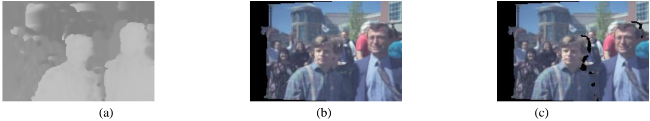
Figure 3: Results of multi-view stereo algorithm: (a) depth estimate for first frame; (b) warped (resampled) images without visibilities; (c) with visibility computation.
