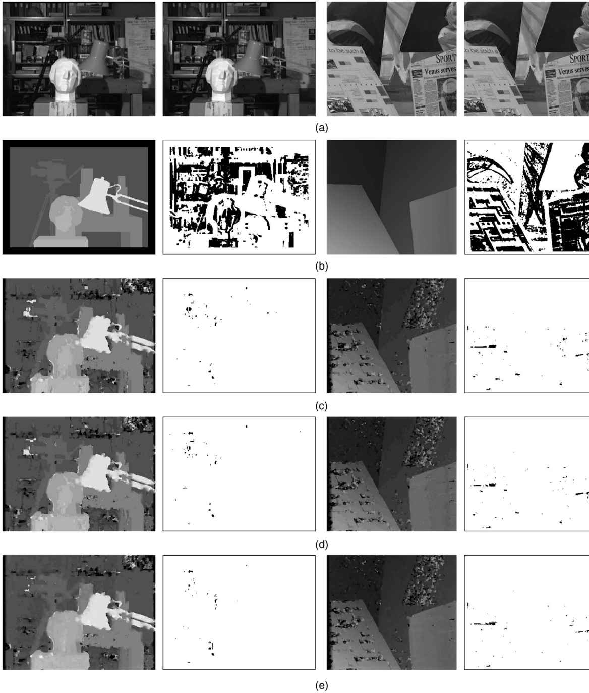
Fig. 4. Test images and selected results. (a) Input images: Tsukuba (left) and Venus (right). (b) True disparity maps and textured nonoccluded regions (shown in black) in which errors are being evaluated. (c) Traditional integer-disparity SSD results (disparity maps and error maps): s = 1 , i = 0 , SD. (d) Birchfield-Tomasi results: s = 1 , i = 0 , BT. (e) Results for half-pixel disparities with symmetric matching and interval difference: s = 2 , i = 1 , ID. The error maps in (c), (d), and (e) show in black the “bad” matches in textured, nonoccluded regions, i.e., pixels whose floating point disparity differs from the ground truth by more than 1.
