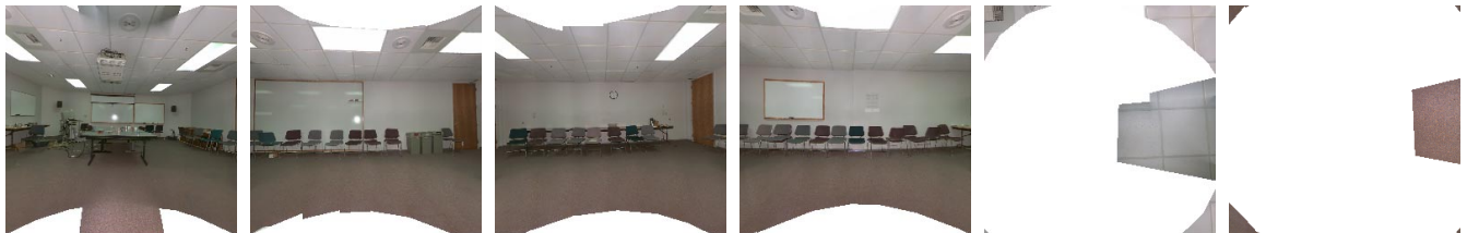
Figure 5: Cubical texture-mapped model of conference room (from 75 images taken with a hand-held digital camera).
