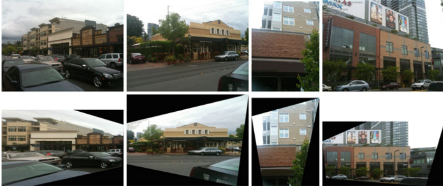
Fig. 15.2 Example query images from a mobile phone camera. The top row shows the original images, while the rectified versions of these images computed using our method are shown the second row
