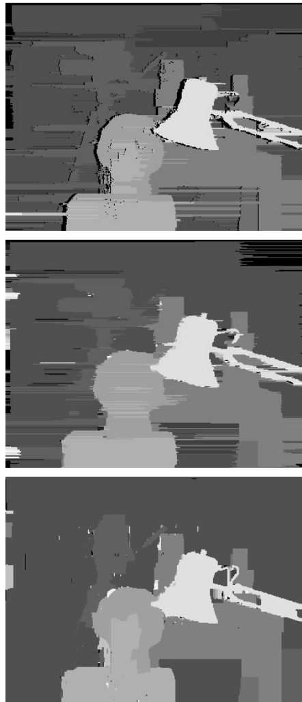
Figure 3: “Best” disparity maps computed by the global algorithms. Top: Dynamic programming (DP), \lambda = 100 , \gamma = 1 , \text{opt\_ocst} = 60 . Middle: Scanline optimization (SO), \lambda = 100 , \gamma = 0 . Bottom: Graph cut algorithm (GC), \lambda = 1000 , \gamma = 2 .
