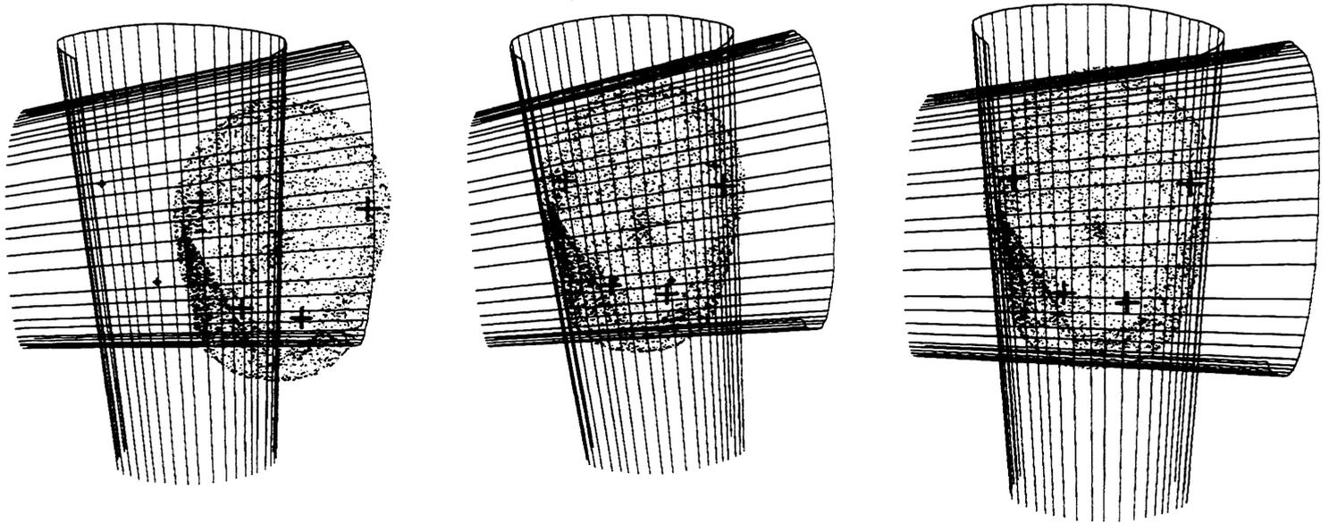
Figure 8: Convergence of 3-D / 2-D algorithm : A set of projection lines issued from a pair of X-rays of the skull converges towards the skull surface segmented on CT images
