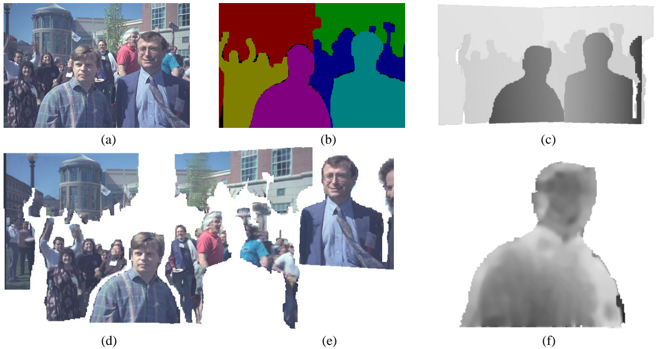
Figure 4: Results on the symposium sequence: (a) third of five images; (b) initial segmentation into six layers; (c) recovered depth map (darker denotes closer); (d) and (e) the five layer sprites; (f) residual depth image for fifth layer.
